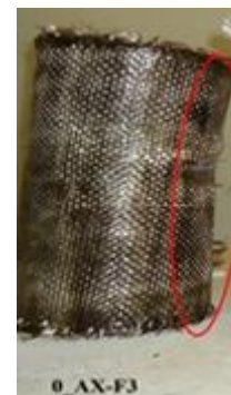
Figure 5. Failure of the sheet at ultimate load
